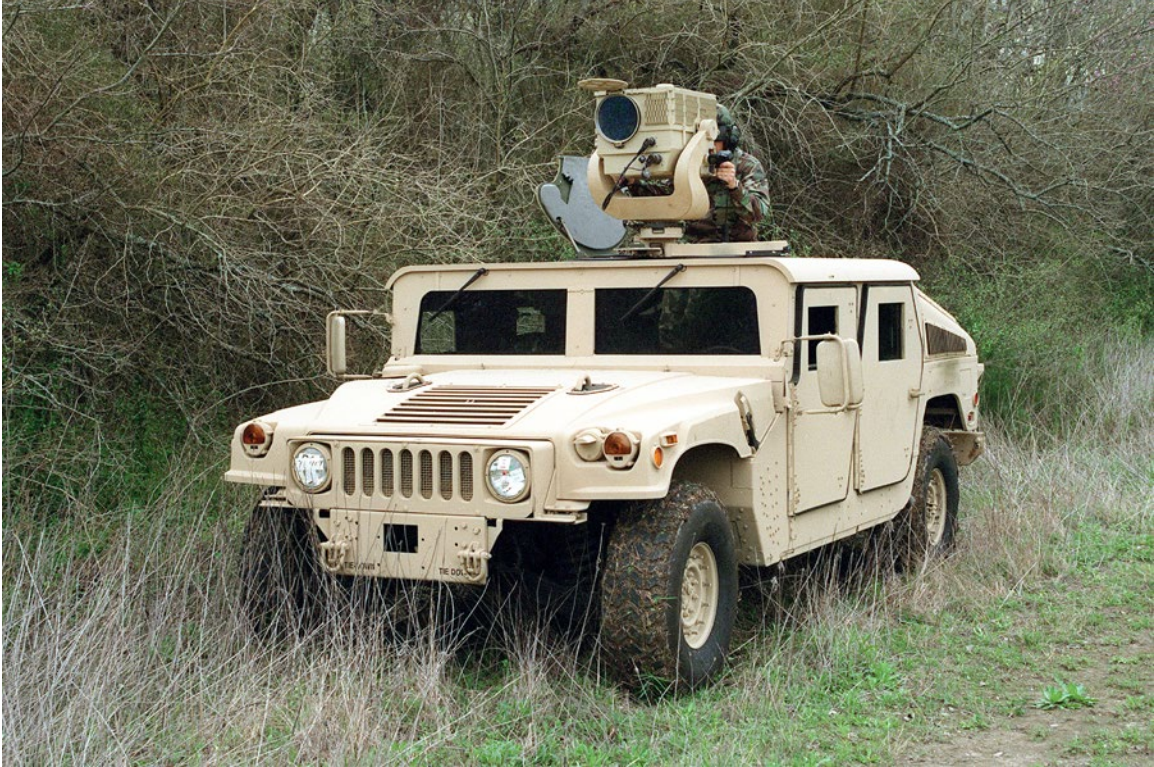
Figure 6. The HMMWV-LRAS3 combination — the essence of a new contact paradigm. (Photo from the U.S. Army Armor Branch archives)
